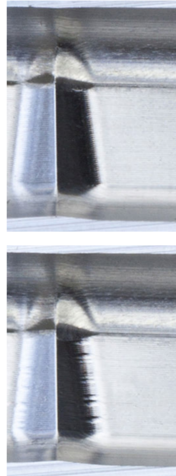
Top figure: part milled with ADP Bottom figure: part milled without ADP
