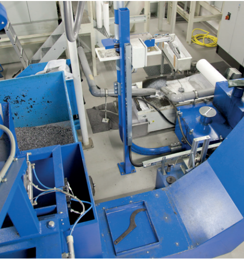
Processing facilities chop metal chips into small pieces and withdraw moisture, thus allowing them to be economically recycled.
