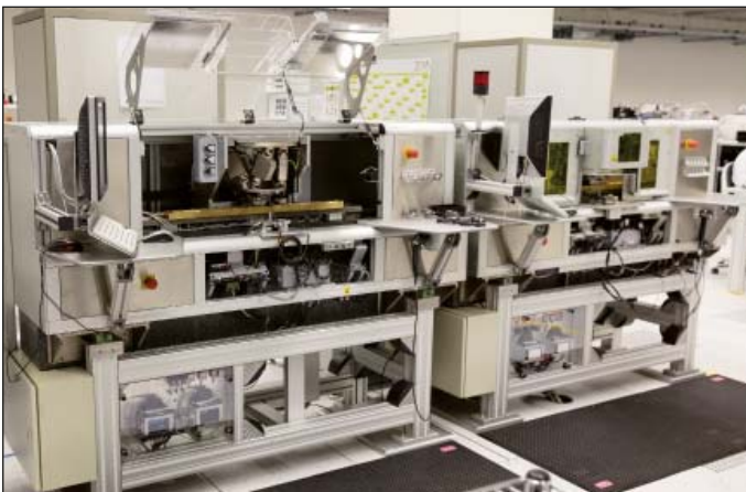
Figure 10: The interpolation deviation of each exposed linear encoder is measured on a special measuring station by measuring the scanning head.
