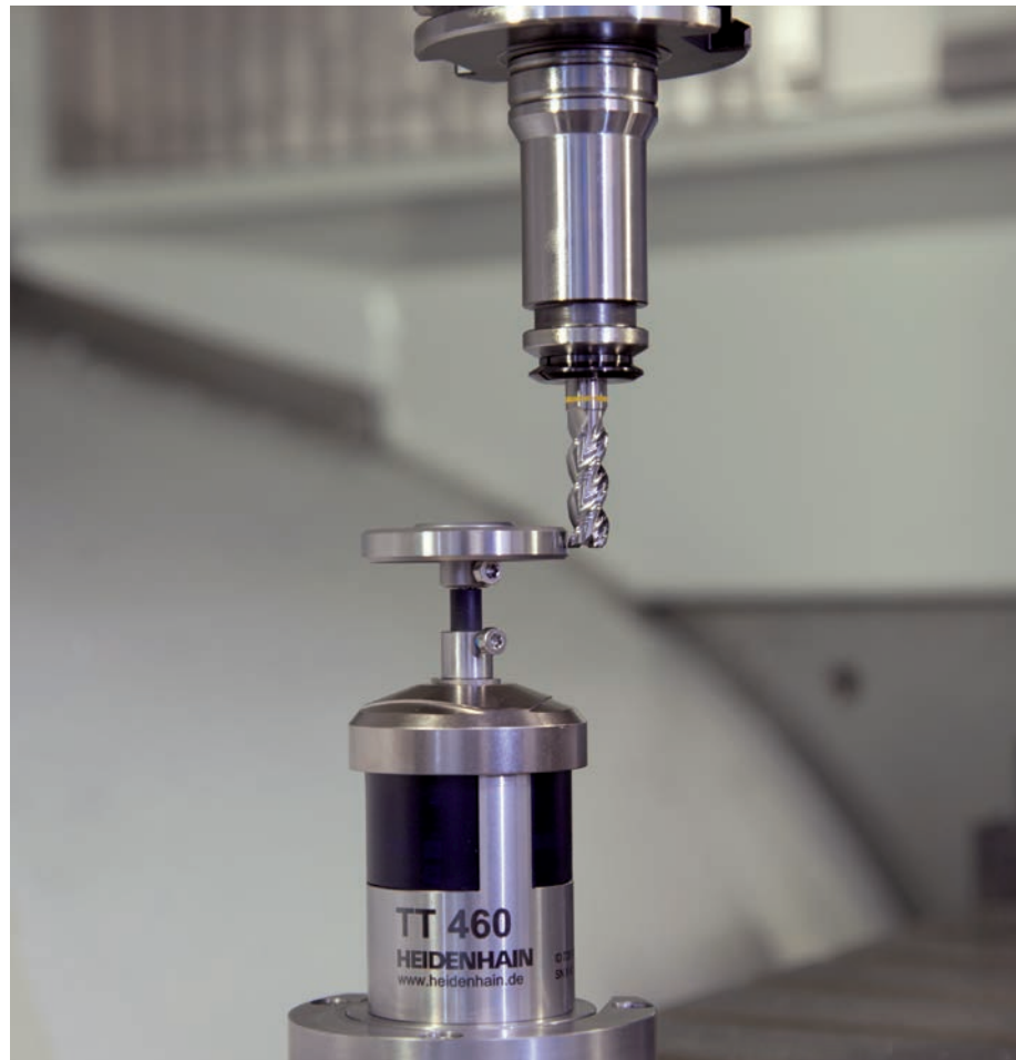
Individual tooth measurement, such as for inspecting indexable inserts (not for brittle materials)
