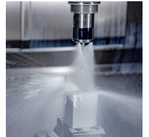
Cleaning with cooling lubricant
