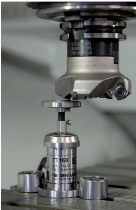
Measuring the tool length
