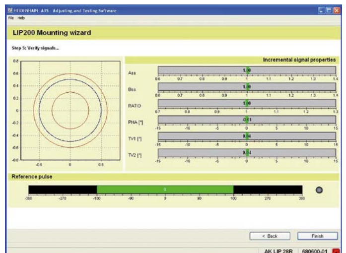
Commissioning using PWM 20 and ATS software
