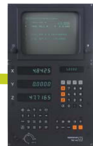
1981: TNC 145, the first contouring control from HEIDENHAIN
